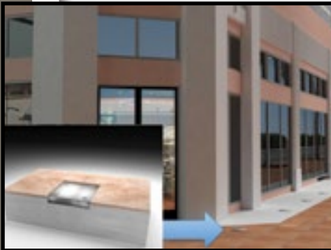
Post inserts are covered over with plates in the side walk. Plate could also be designed to aesthetically disappear.
